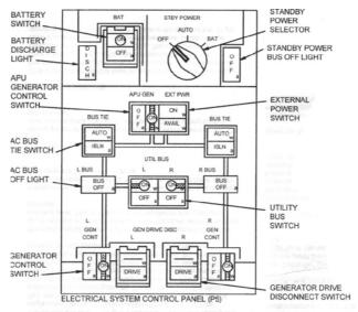
Flight Deck Electrical System Control Panel
