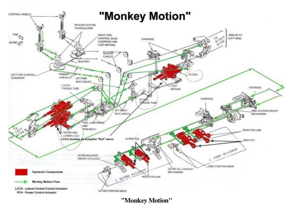
Pitch Control: Dual System, not nearly as complicated as the Lateral Control System. The Captains column controls the left elevator PCA, the First Officers column controls the right PCA. These two independent systems are normally bussed together, but there is an override system and either one can control the elevators fully in the event that one fails.
