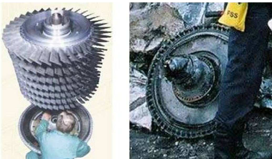
Comparison of intermediate pressure compressor stages on the RB211 to the wreckage
