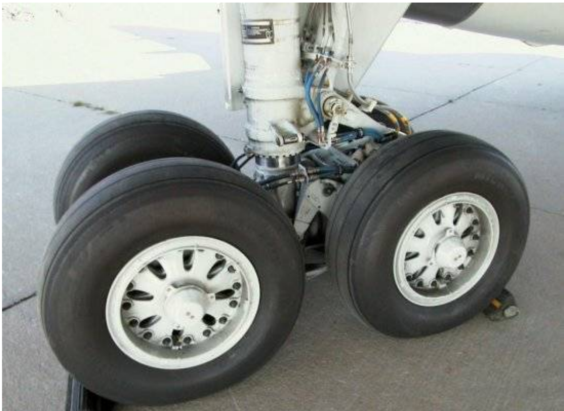
Boeing 757-200 main landing gear wheels with 8 cutouts
