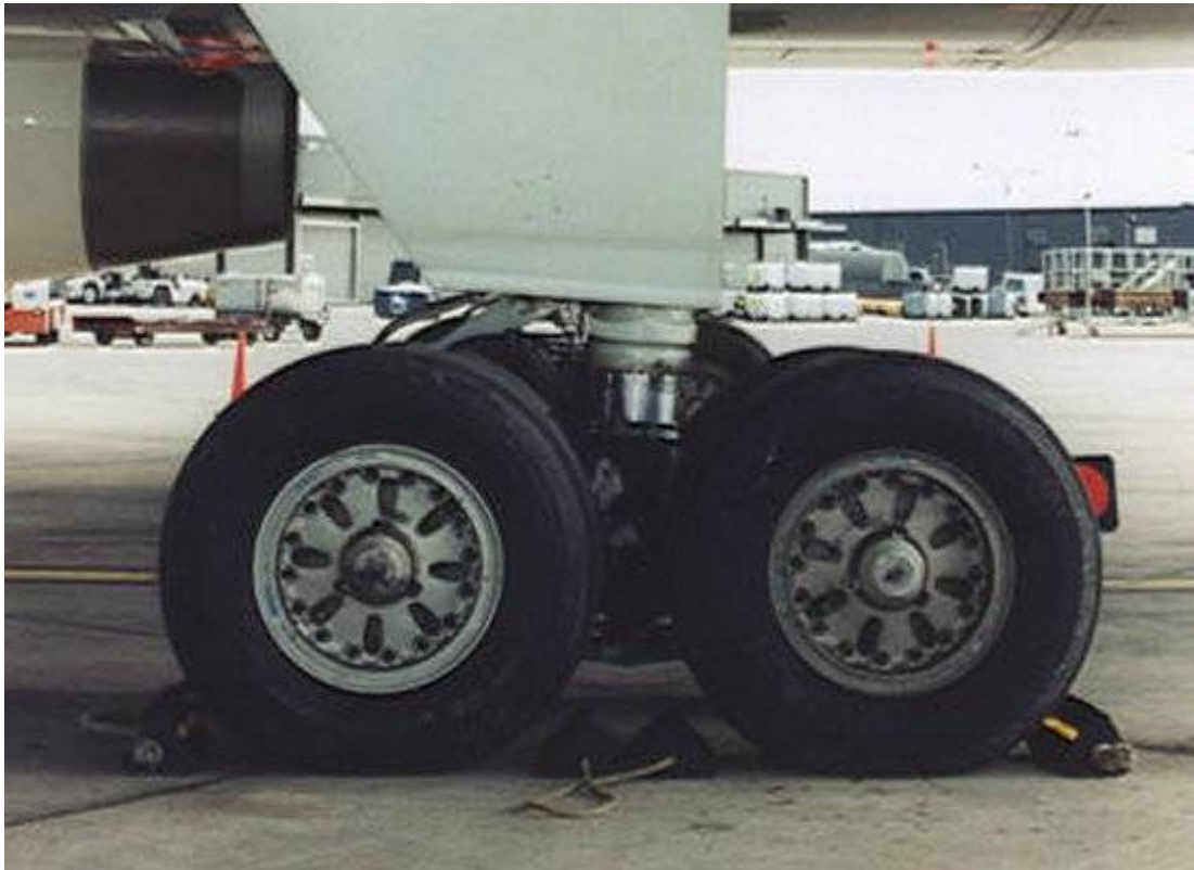
Boeing 757-200 main landing gear wheels with 8 cutouts
