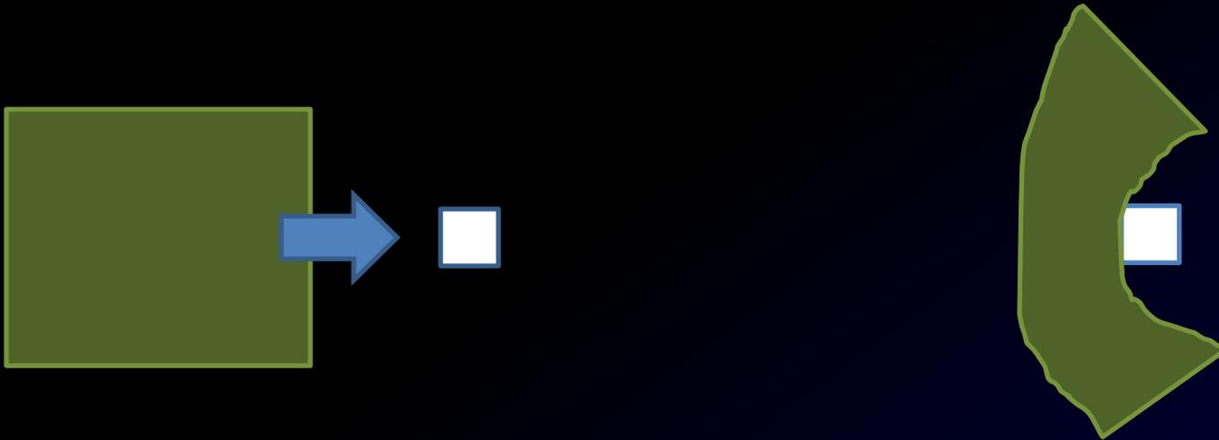
**Case 3:** Flexible impactor deforms until it stops or breaks
