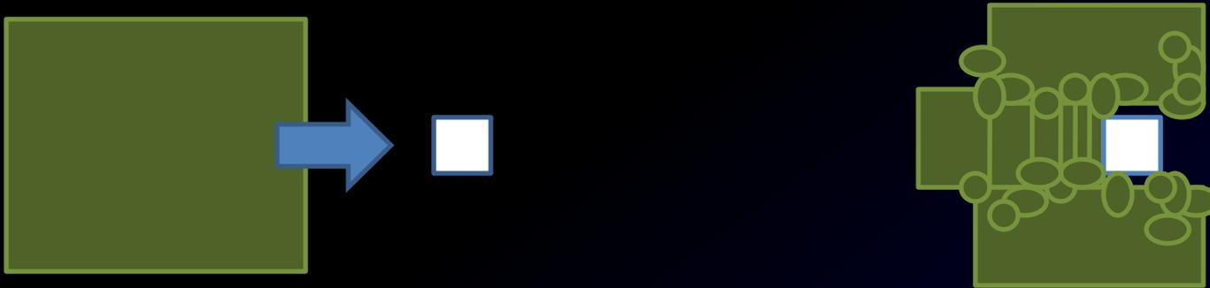
**Case 2:** Brittle impactor jars impacted object, then fractures
